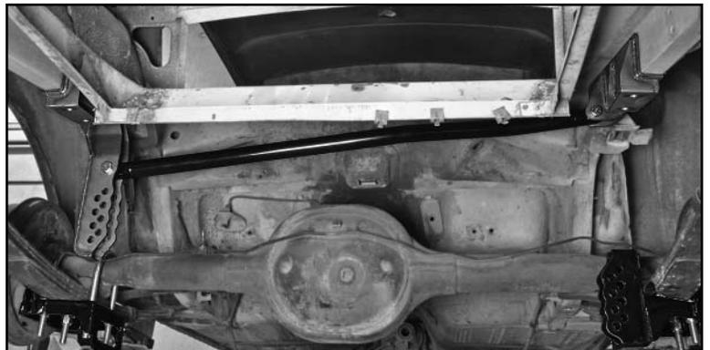
19. Thread the jam nut onto the rod end until there are 4-5 threads above the nut.
