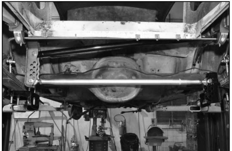
23. Secure using 1/2" x 2-1/2" bolt, two flat washers, two 1/4"-thick misalignment spacers, and locknut. Tighten to 60 lb-ft.
