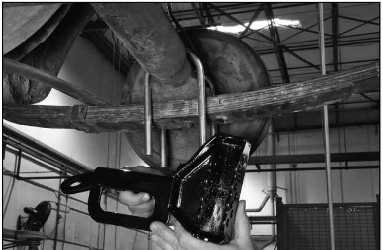
In addition to factory shock mount, the passenger-side spring plate features multiple adjustment holes for the panhard bar, the anti-roll-bar endlink mount, and a tie-down loop.
