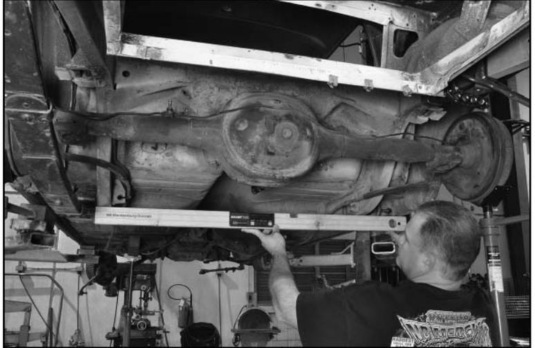
6. Position the passenger-side frame bracket 17-1/16" forward of the inside edge of rear spring-bushing sleeve.
