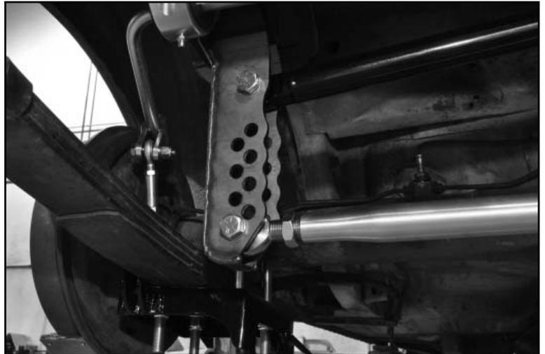
22. The opposite end of the panhard bar must be installed at the hole on the axle bracket that positions the bar closest to level. Rotating the radius rod will lengthen or shorten the bar as needed. Do not rotate the free rod end with the radius rod.
