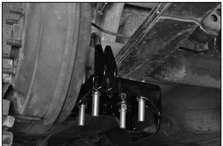
The bent end of the welded support tube mounts to the passenger-side frame bracket. The tube must be rotated so that it jogs away from the rearend housing. Refer to the assembly diagram for clarification.
