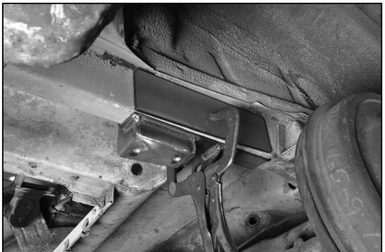
8. Mark the bracket and support strap outline onto the frame rail.
