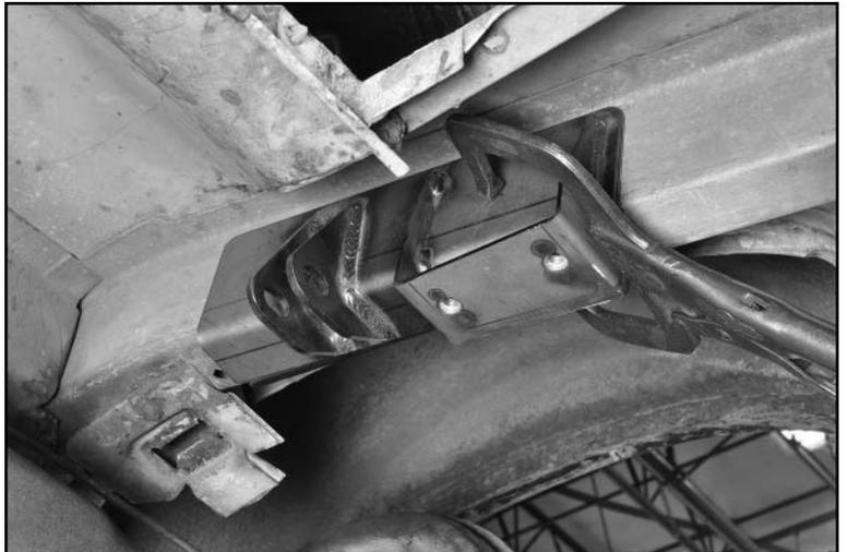
11. Make sure the anti-roll bar pads are level to the ground, then tack weld the bracket and strap to the rail.
