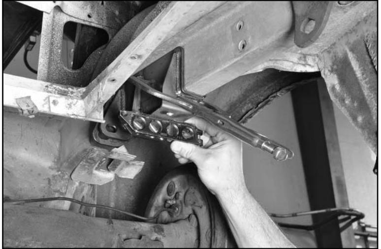
12. Use the same position measurement of 17-1/16" for the driver-side bracket. Follow the same weld-prep procedure.
