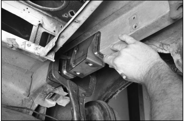
9. Use a scotch-brite pad to remove any paint or coating material along the weld area.
