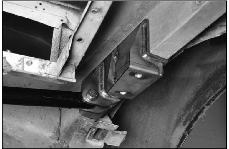
17. Secure driver's side end of support tube to uppermost hole on bracket using 1/2" x 2-1/2" bolt, two flat washer, two 3/16"-thick spacers, and locknut. Tighten to 60 lb-ft.
